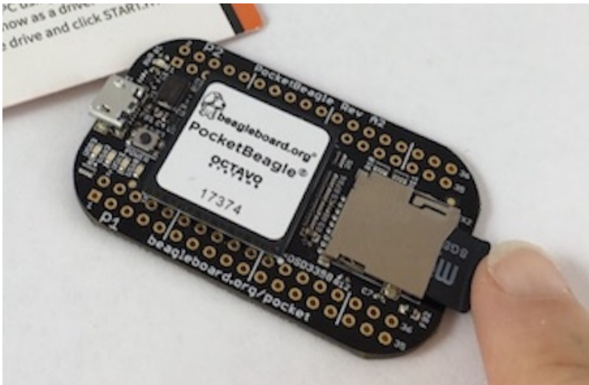
Fig. 3.10: Insert the microSD Card into PocketBeagle
