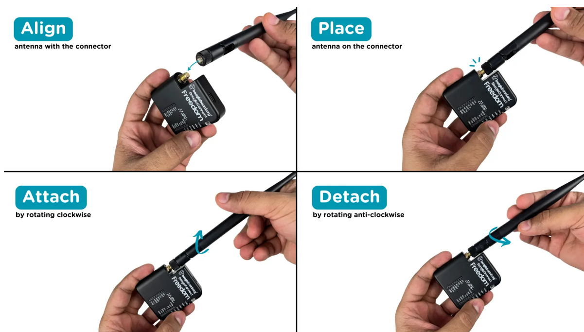
Fig. 2.2: Attaching antenna to BeagleConnect Freedom
