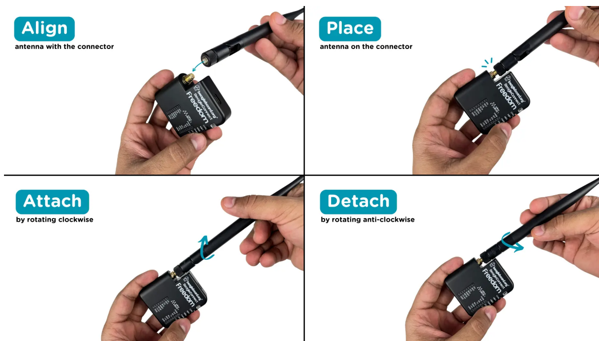
Fig. 2.2: Attaching antenna to BeagleConnect Freedom
