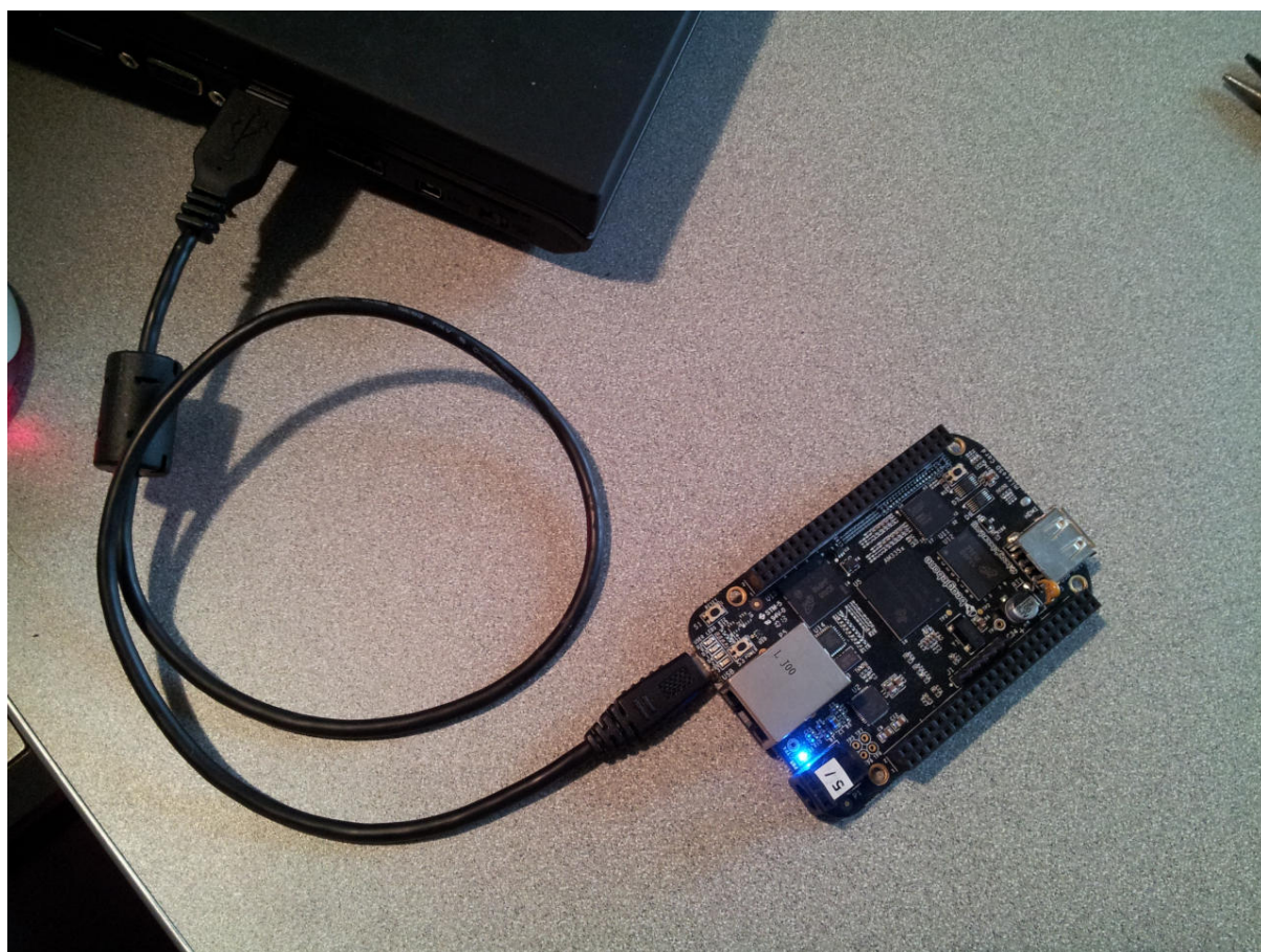
Fig. 1.1: Plugging BeagleBone Black into a USB port
