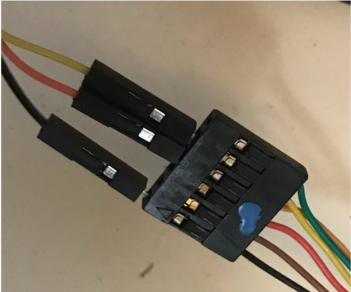
Fig. 5.6: JST to FDTI connection
