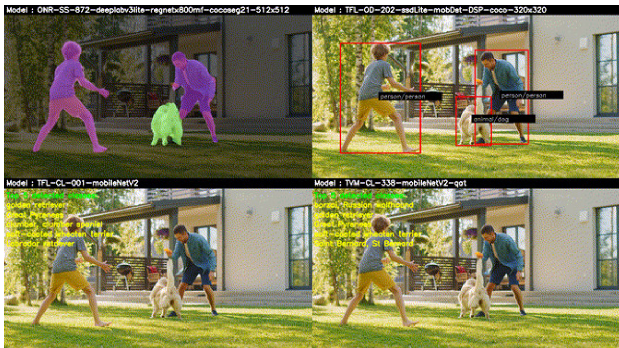
Fig. 5.4: Sample output showing single input, multi-inference output
